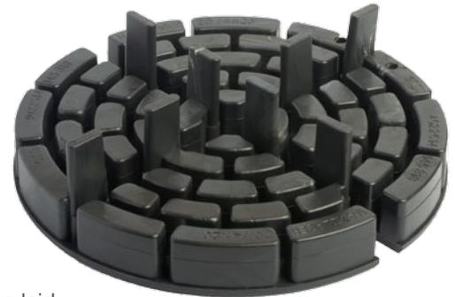
**Application:** Laying paving slabs on waterproofed flat roofs or on concrete surfaces WITH NO slope. The slabs must be laid with a protective layer between the waterproof seal and the pedestal support made of at least 200 g/m<sup>2</sup> raw glass fibre matting.
